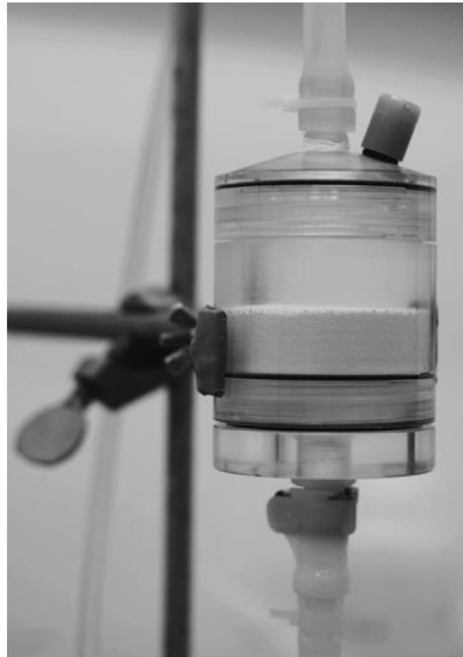
Fig. 1 Column used for concentration of cesium from 100 seawater (internal diameter 42 mm, 25 mL of AMP-PAN)
