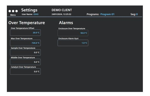
The *Settings* screen allows the user to set the over temperature offset and Enclosure over temperature alarm for the Pyrolyser
