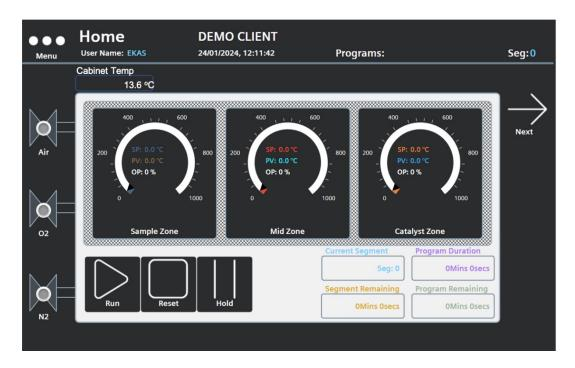
The **HOME** screen provides an overview of the Pyrolyser-6 Trio GenIV, it displays all the temperature and profile information. The 3 heating zones are visually displayed, indicating their current SP, PV & OP%. In the correct Log In Mode pressing on the centre any of the zones will take you to the relevant settings for this zone, see section 5.2 for more details on PID settings.
