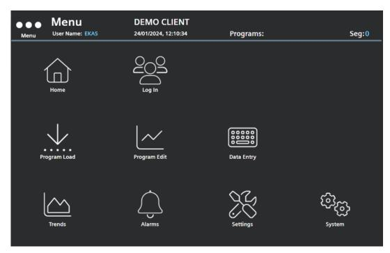
The Menu screen provides the access to all the sub screens on the HMI.
