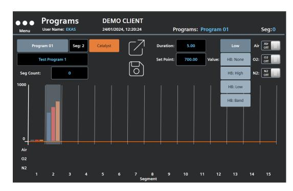
The **Program Edit** screen is divided into 2 parts, the upper part provides the user with the relevant options for the program name and segments. The lower part provides a graphical overview of the profile, segments and the gas supply solenoids that are active.
