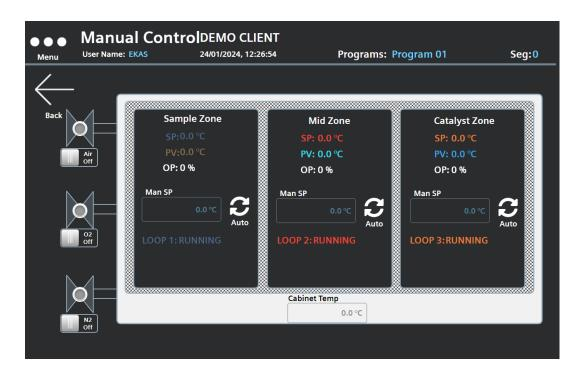
The MANUAL Control screen provides a similar overview to the MAIN screen, however it also provides the user with some manual options for operation of the Pyrolyser outside of a predefined programme.
