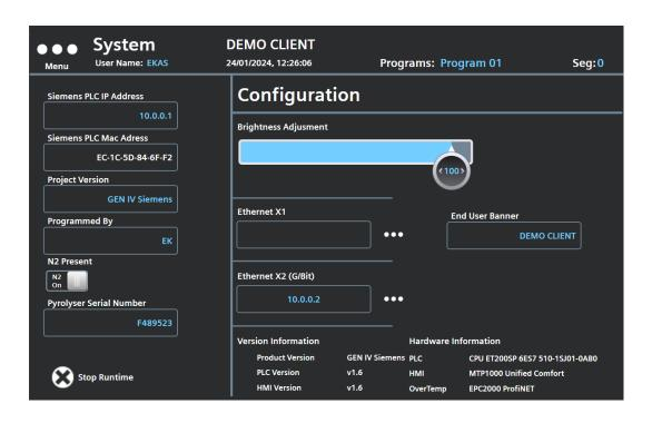
The *System* page provides basic information about the system (IP / MAC address of the PLC, Project version and software version information, System Serial No.). The page also allows users to adjust the display brightness and enter a User Banner (e.g. Company Name).
